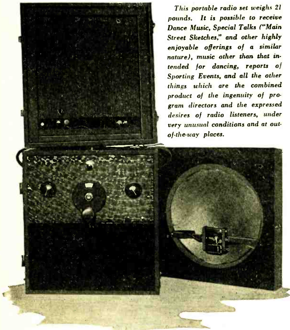
Photograph of portable receiver designed to include the new screen grid tube. As the current drain of this tube is slight, it lends itself well to use in receivers such as this one.
